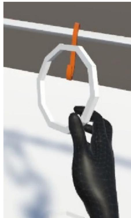
Once a grasping action is detected the mesh of the hand is blocked at the last known state.
