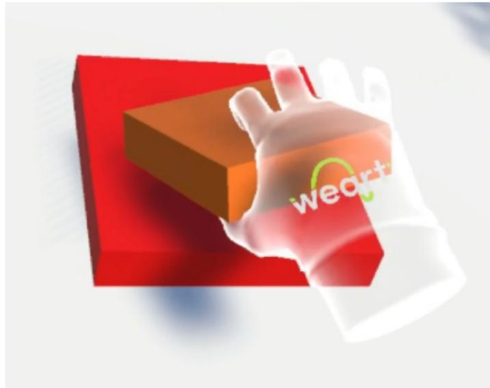
Once a collision is detected the system locks the finger to prevent it from closing beyond the point of contact and the grasping event can begin.
