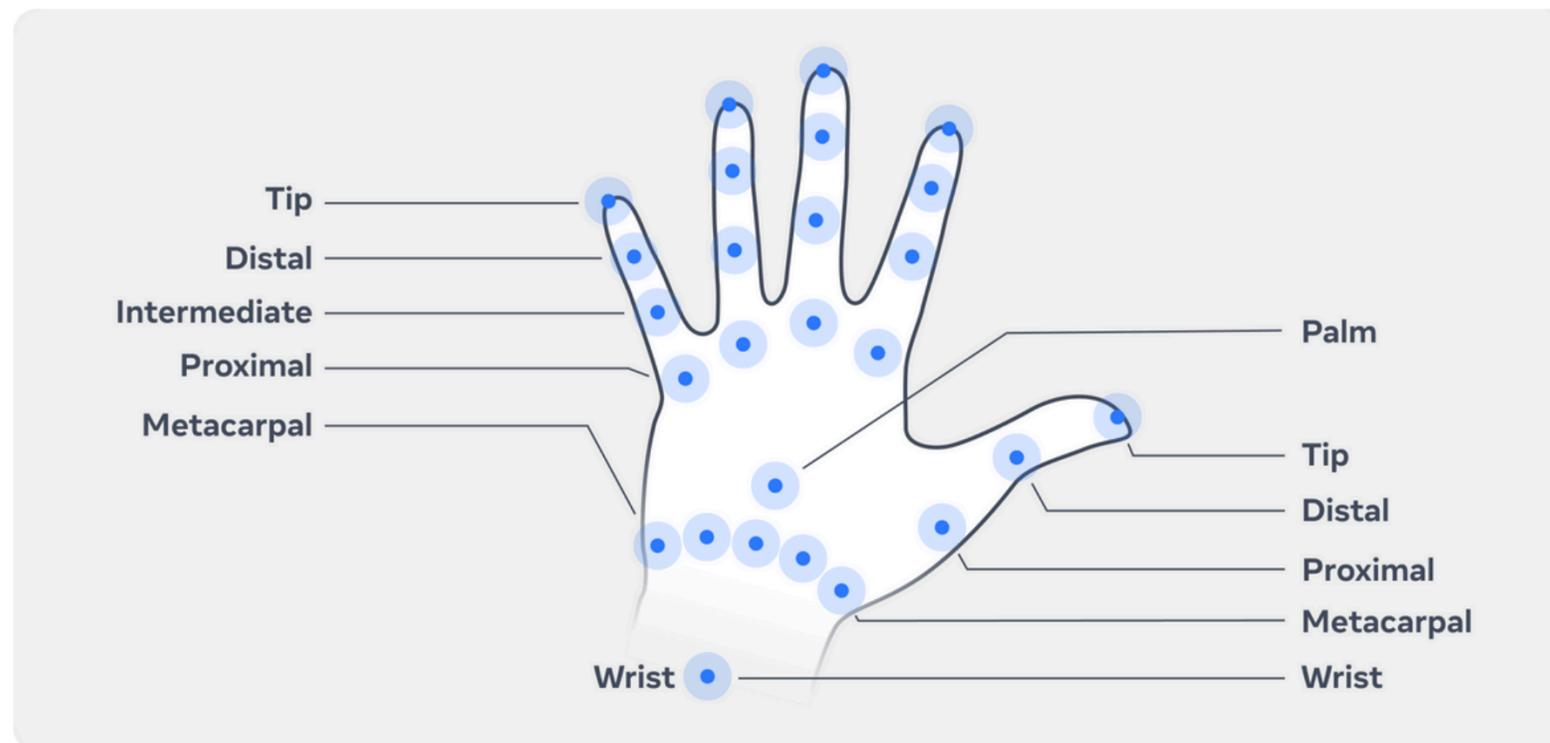
The SDK provides a computer vision model to estimate the pose (position and rotation) of different bones and joints of the hand.
