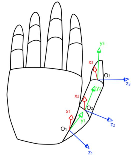
The controller features a term proportional to the error in cartesian space and a Jacobian null-space term to keep the joints within the  $[0, \pi/2]$  limit.
